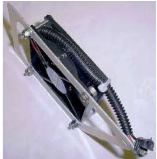
Figure 7 - Fan Mounted to G10 Bracket
